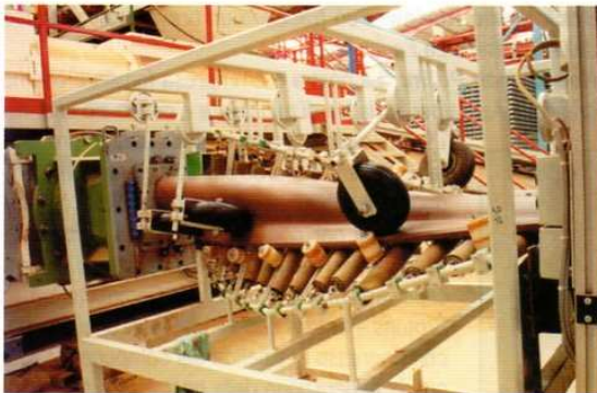
Stage of extruding pre-shaped bats with double vertical exit Fase di estrusione gallette presagomate in doppia uscita verticale
