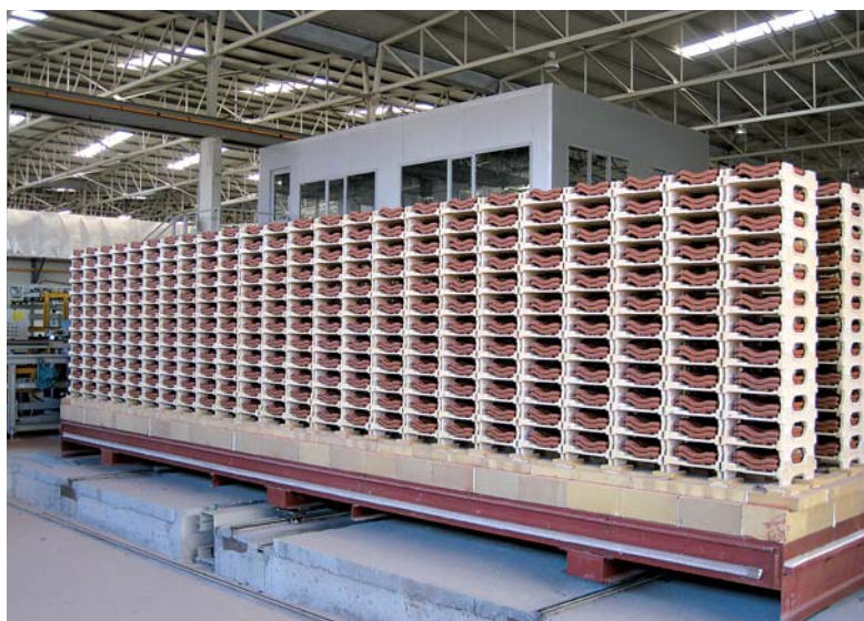
Carro forno con materiale cotto. A kiln car loaded with fired roof tiles.
