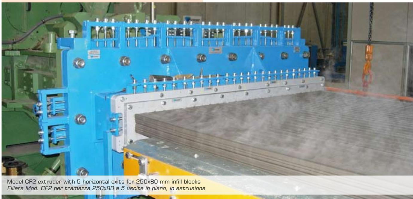
Model CF2 extruder with 5 horizontal exits for 250x80 mm infill blocks
