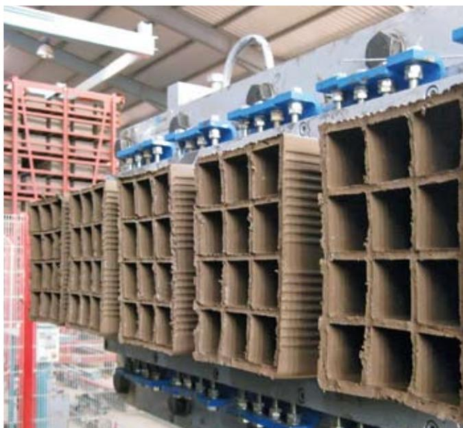
Thrust tests: 5-exit die B12 150x200
