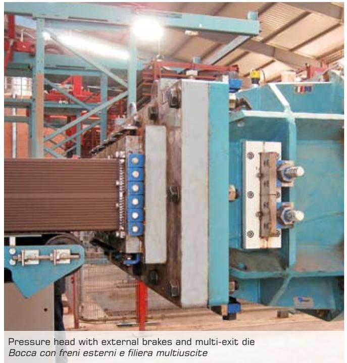
Pressure head with external brakes and multi-exit die
