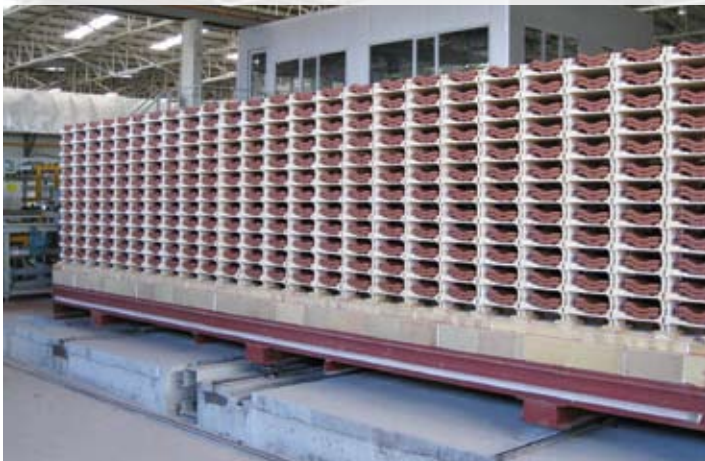
Kiln car with fired material Carro forno con materiale cotto
